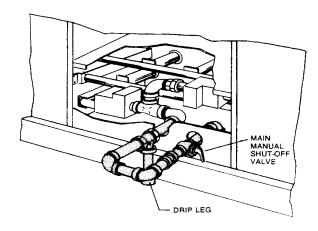
FIGURE 7 - BOTTOM SUPPLY CONNECTION EXTERNAL SHUT-OFF
